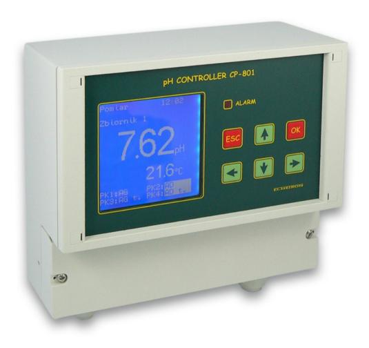
The device is easy to operate, has an English menu. It is equipped with a collective optical signalisation of correct working and the progress of regulation process.
